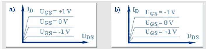
Match the transfer characteristics in figure to corresponding MOSFET type
