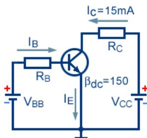
What is collector-emitter voltage  $U_{CE}$  for transistor in figure?
