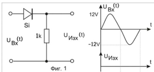
Draw the ac output voltage waveforms for the circuit in figure.
