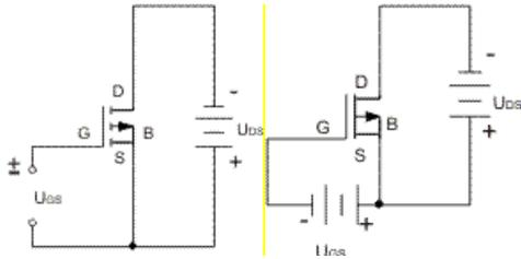
What is the correct output characteristic for *P*-channel depletion-mode MOSFET? (or for *N*-channel depletion-mode MOSFET?)
