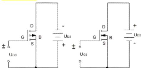
What is the correct schematic of a depletion- mode P-channel MOSFET? / (or of an enhancement- mode P-channel MOSFET?)
