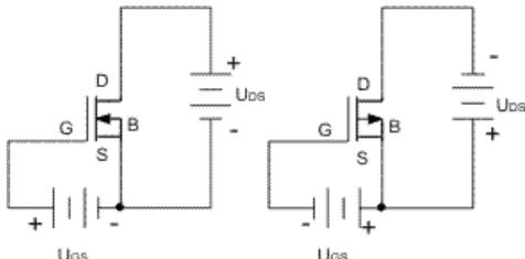
What is the correct schematic of an enhancement mode P-channel MOSFET? / (or of an enhancement- mode N-channel MOSFET?)
