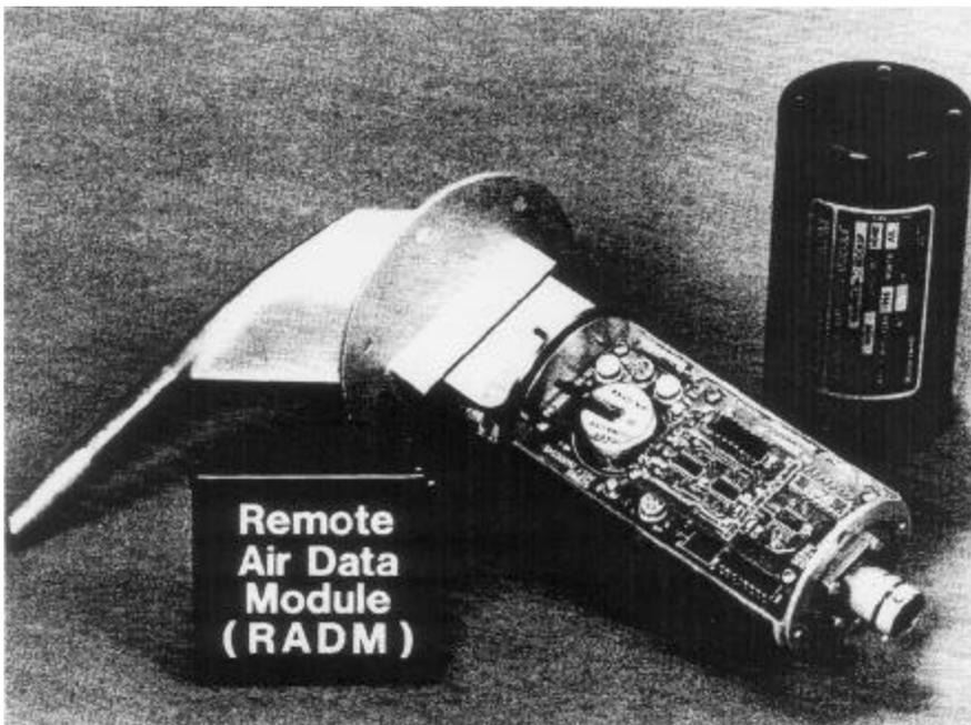
**COMPLETE PRESSURE-TRANSDUCER SYSTEM** is mounted on a pitot tube that extends into the air stream flowing past a moving aircraft. The transducer is used in two applications; one is measuring the static, or ambient, pressure, and the other is monitoring the dynamic pressure associated with the aircraft's velocity. The module is now being flown aboard Boeing's next-generation-technology demonstrator aircraft.
