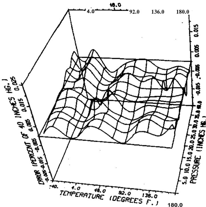
ACCURACY OF THE TRANSDUCER is vastly improved by an algorithmic process called modeling that compensates for temperature-dependent errors and nonlinearities in the "raw" sensor data. The vertical scale in this illustration is magnified 2,000 times in order to make slight departures from the ideal sensor response visible. The graph indicates that for all combinations of pressure and temperature measured the transducer is accurate to within  $\pm 0.01$  percent.
