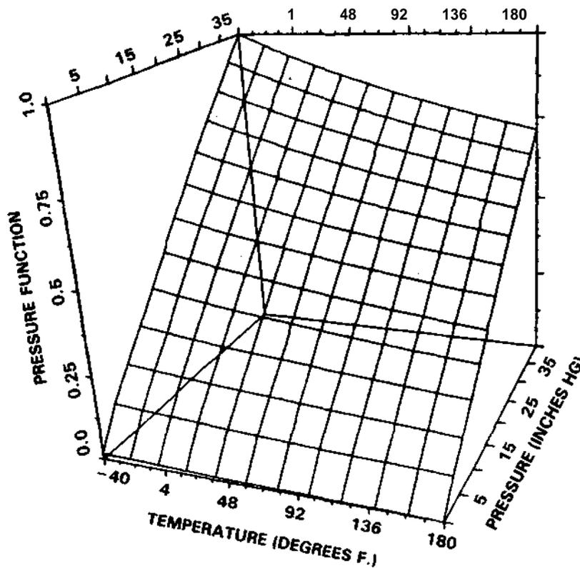
UNCOMPENSATED OUTPUT of the sensor depends strongly on temperature as well as pressure. The fact that the surface of the graph slopes downward to the right indicates that the sensor becomes less sensitive to pressure as the temperature increases. There is also a slight nonlinearity in the response of the sensor to pressure at a fixed temperature.
