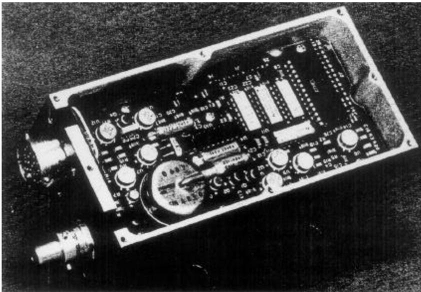
**AIR-DATA MODULE** for the Aerospatiale Airbus A320 is similar to the one shown in the previous illustration but is not mounted on a pitot tube. Eight of these modules are installed in each Airbus, providing pressure measurements for the Honeywell Air Data Inertial Reference System.
