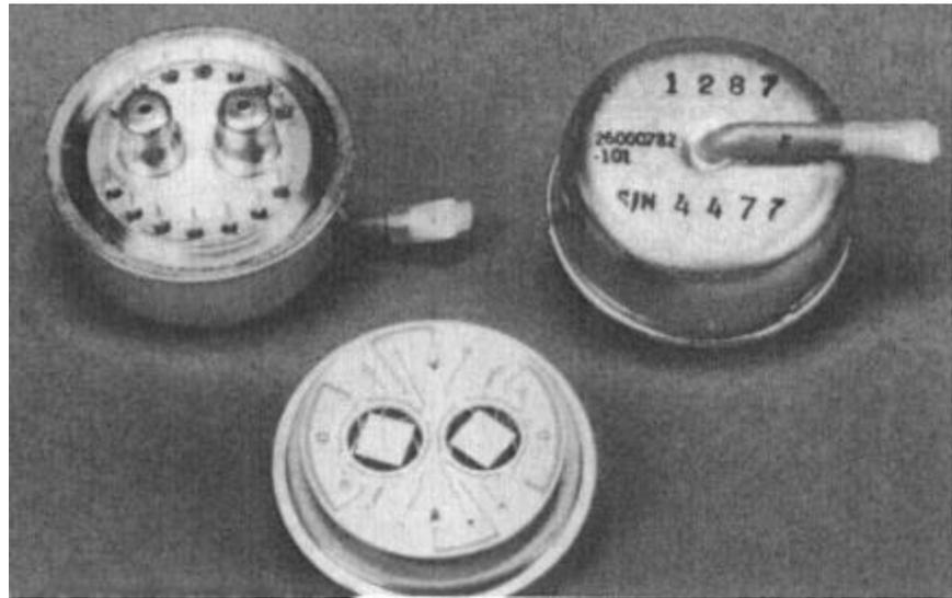
**QUASI-DIFFERENTIAL SENSOR** for air-data applications measures two absolute pressures with high precision in order to synthesize a differential measurement. Mounting the two sensors in the same housing, so that they share the same reference vacuum, eliminates a potential source of error, namely differences in the residual pressures of two independent reference-vacuum chambers.
